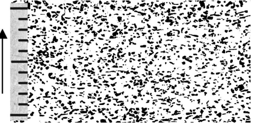
FIG. 3. Microstructure of snow type tested. Binarized picture of a surface section. Black denotes ice, white is the pore space ( \rho = 250 \text{ kg m}^{-3} ). Scale given is 1 cm. Arrow points to the snow surface (top margin was parallel to the snow surface).
